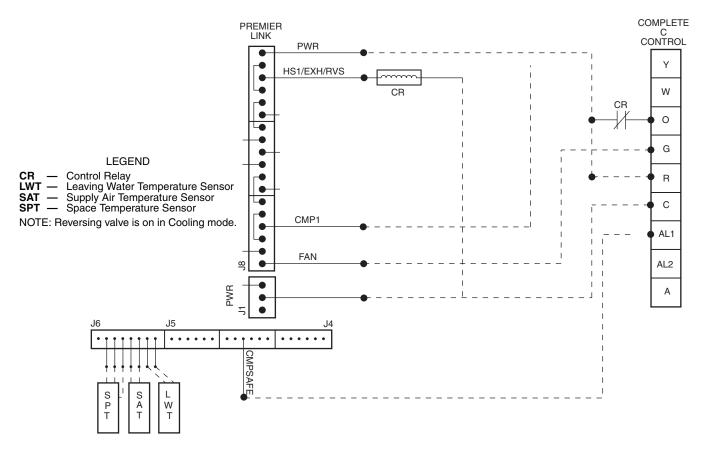
Fig. 23 — PremierLink™ Controller Applications with Complete C Control
